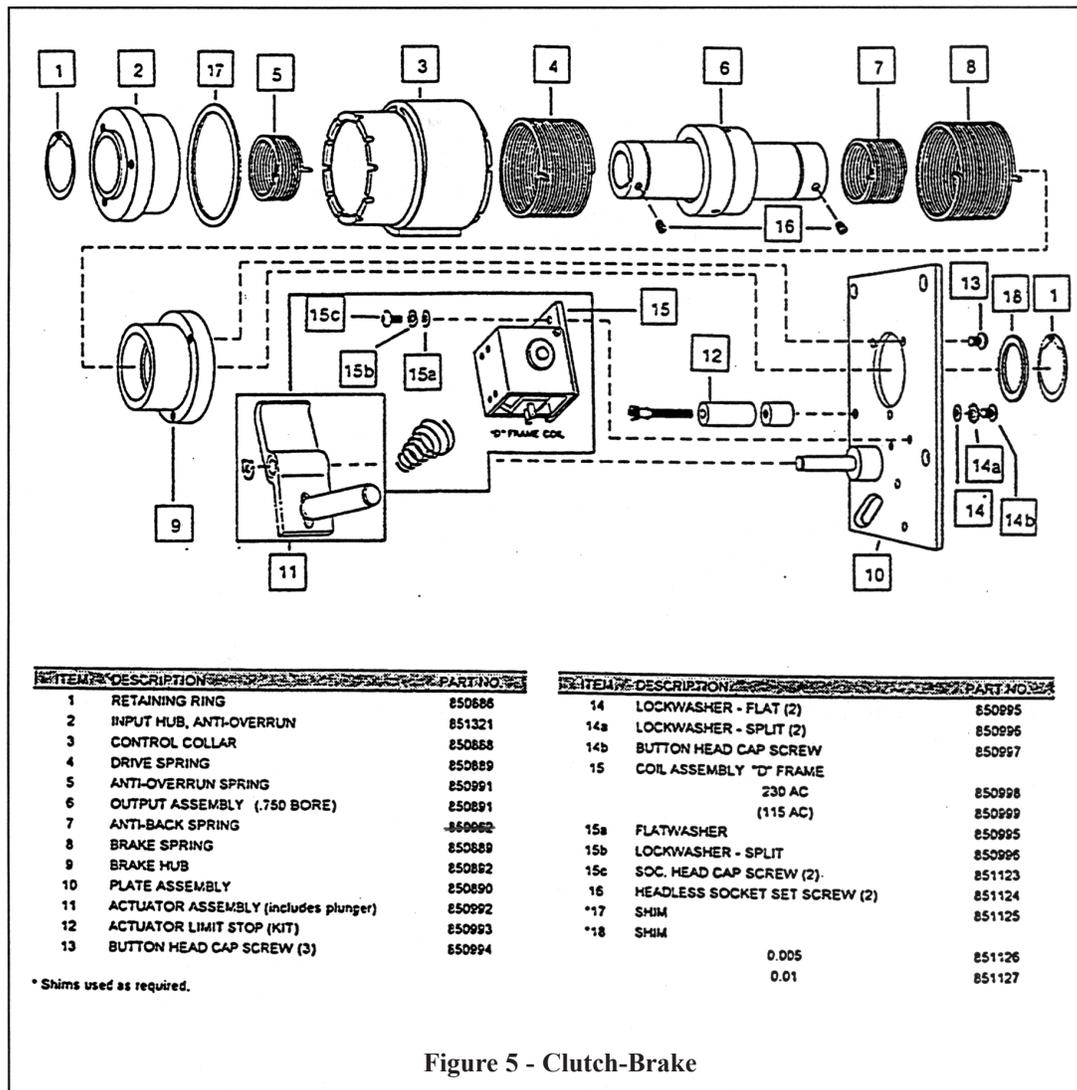
Figure 5 - Clutch-Brake
