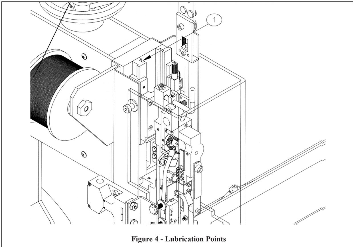
Figure 4 - Lubrication Points
